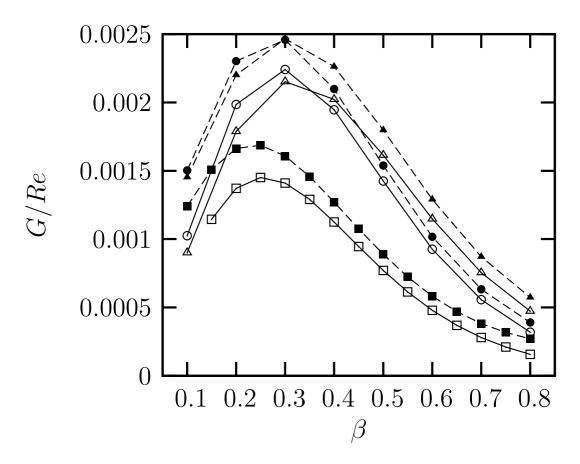
Objective function G/Re: effect of  $x_{\rm in}$  and  $\beta$  and norm choice (PEN vs. FEN) for M=3,  $T_w/T_{\rm ad}=1$ ,  $x_{\rm out}=1.0$ .  $\Box$ ,  $x_{\rm in}=0.0$ ;  $\circ$ ,  $x_{\rm in}=0.2$ ;  $\triangle$ ,  $x_{\rm in}=0.4$ .  $\Rightarrow$  Up to 60% difference for  $x_{\rm in}=0.4$  and  $\beta=0.1$ .
