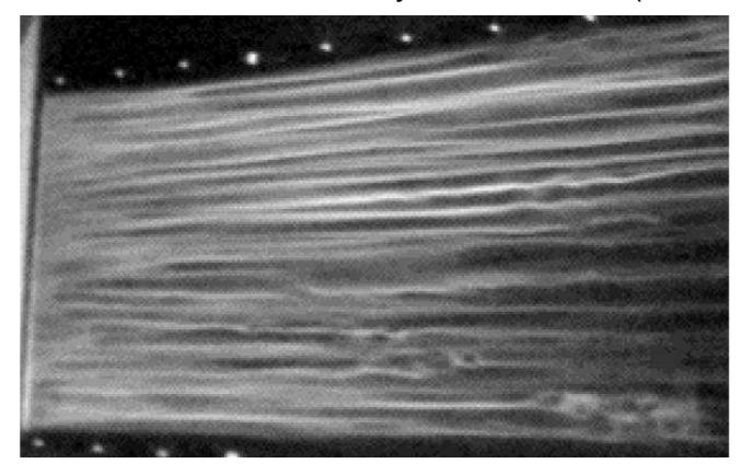
...streaks (instead of waves) can develop where the flow is stable according to the classical neutral stability curve. Alternative mechanism to TS waves: Transient growth.
