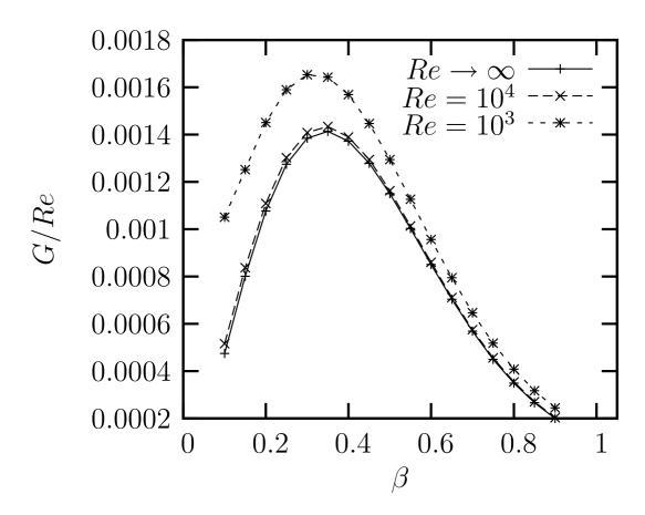
Objective function G/Re: effect of Re and  $\beta$  for M=3,  $T_w/T_{\rm ad}=1$ ,  $x_{\rm in}=0$   $x_{\rm out}=1.0$ , FEN.
