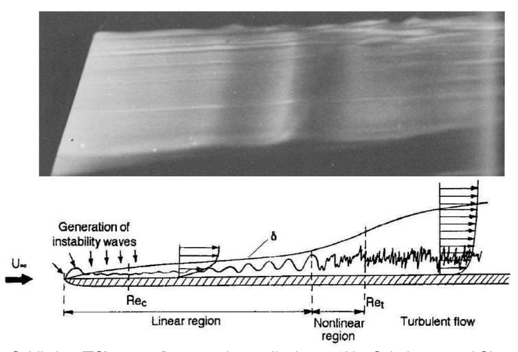
Tollmien-Schlicting (TS) waves first experimentally detected by Schubauer and Skramstad (1947), "Laminar boundary-layer oscillations and transition on a flat plate", *J. Res. Nat. Bur. Stand* 38:251–92, originally issued as NACA-ACR, 1943.
