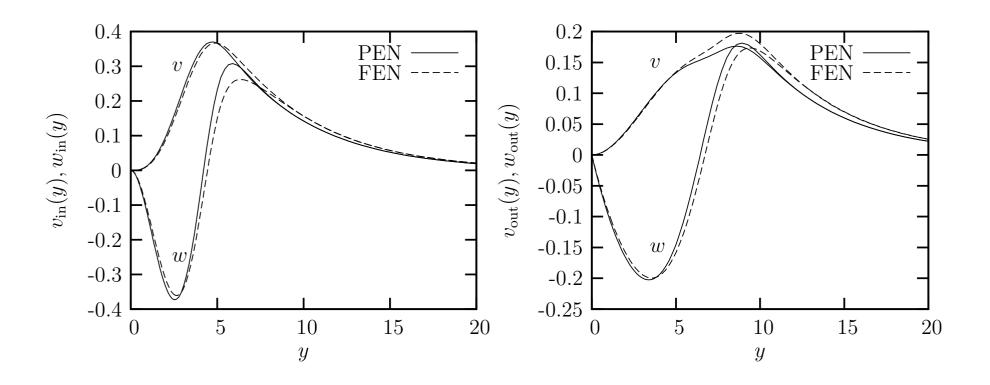
Inlet and outlet profiles: effect of norm choice (PEN vs. FEN) for M=3.0,  $Re=10^3$ ,  $x_{\rm in}=0.4$ ,  $x_{\rm out}=1.0$  and  $\beta=0.1$ .
