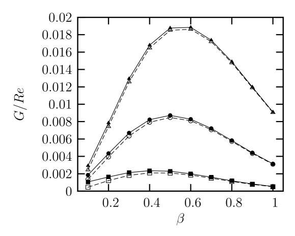
Objective function G/Re: effect of  $\beta$ ,  $T_w/T_{\rm ad}$  and norm choice (PEN vs. FEN) for M=0.5,  $Re=10^3$ ,  $x_{\rm in}=0$   $x_{\rm out}=1.0$ .  $\Box$ ,  $T_w/T_{\rm ad}=1.00$ ;  $\bigcirc$ ,  $T_w/T_{\rm ad}=0.50$ ;  $\triangle$ ,  $T_w/T_{\rm ad}=0.25$ .  $\Rightarrow$  No remarkable norm effects; cold wall destabilizing factor.
