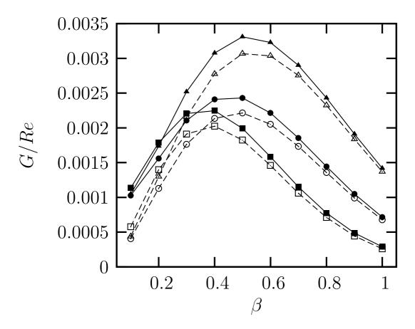
Objective function G/Re: effect of  $\beta$ ,  $T_w/T_{\rm ad}$  and norm choice (PEN vs. FEN) for M=1.5,  $Re=10^3$ ,  $x_{\rm in}=0$   $x_{\rm out}=1.0$ .  $\Box$ ,  $T_w/T_{\rm ad}=1.00$ ;  $\bigcirc$ ,  $T_w/T_{\rm ad}=0.50$ ;  $\triangle$ ,  $T_w/T_{\rm ad}=0.25$ .  $\Rightarrow$  Shift of the curves maximum, enhanced difference between norms ( $T_w/T_{\rm ad}=1.00$ ).
